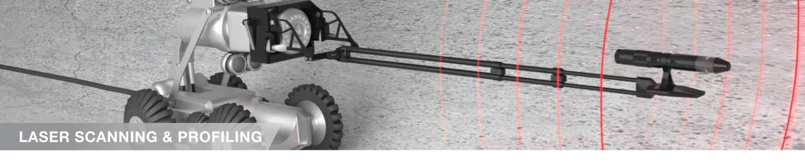
Pipe Hawk Utility Managements iPek laser profiling system provides computer generated pipe profile data. The laser profiler assesses the condition of a pipe by measuring the internal diameter, ovality and capacity of a length of pipeline.
