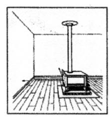
Side and Rear Wall Clearance for an Uncertified Stove - The manufacturer's installation instructions specify the right clearances for the appliance. The clearances for certified appliances vary, but are less than those shown in the following table (from CSA B365) for uncertified appliances. Many of the new, certified appliances have heat shields on the sides and rear, reducing clearances by as much as 90 percent.
