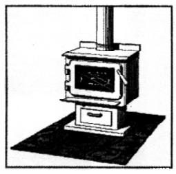
Non-combustible Floor Pad Size and Type – The floor pad protects flooring from hot embers or ashes that might fall from the stove as you fill it or tend the fire. The pad must extend at least 20 cm (8 in.) beyond the sides and rear, and 45 cm (18 in.) in front of the loading door. Also, the floor pad must be a continuous, non-combustible surface. Do not mount the floor pad on carpet, unless the pad is strong enough to resist bending or cracking.
