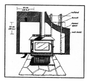
Cut-away of Wall Shield Assembly - By allowing air to flow between the shield and the combustible surface, a wall shielding assembly can safely reduce minimum clearances. The shield must extend at least 50 cm (20 in.) above the top of the appliance and 45 cm (18 in.) beyond each edge of the appliance.
