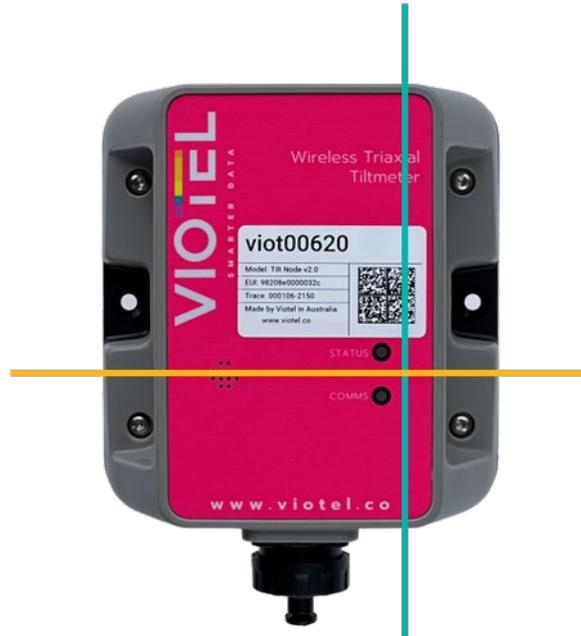
Figure 2 Photo highlighting location of the magnet for TILT-V2.0-INT
