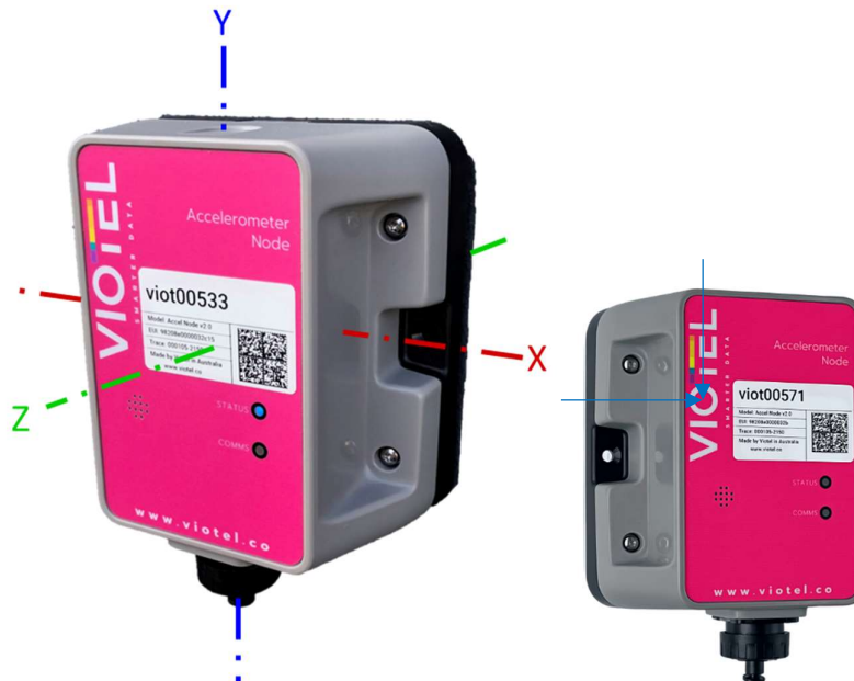
Figure 2 Photo showing X, Y, Z Axis Orientation & Magnet Location
