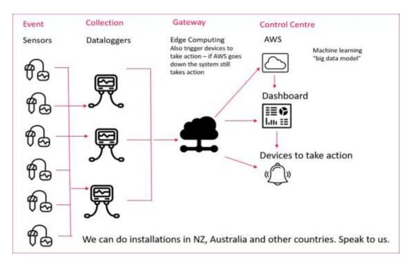
Data are stored within the station and also streamed to the cloud using either mobile phone/data (low-power CatM1), LoRa or satellite networks. Viotel's cloud platform has been built in partnership with Amazon Web Services, using high security certificate exchange to validate connections and encrypted data flows.
