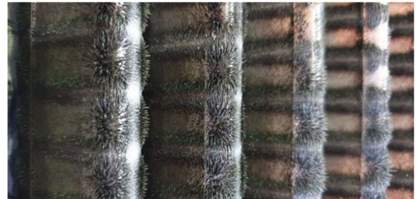
Ferrous material from normal operation trapped on a Mag-Shield® in the hydraulic reservoir of a CAT 994H.
