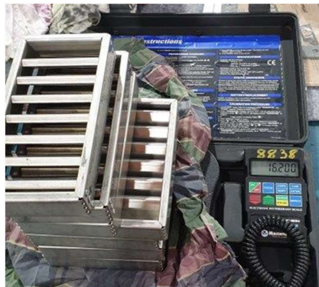
Clean MAG-SHIELD® indicating 110 grams of ferrous material contamination (16.20 kg)
