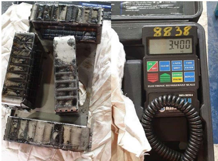
MAG-SHIELD® After 5154 Hours of Normal Operation (No Failure) (3.4 kg)
