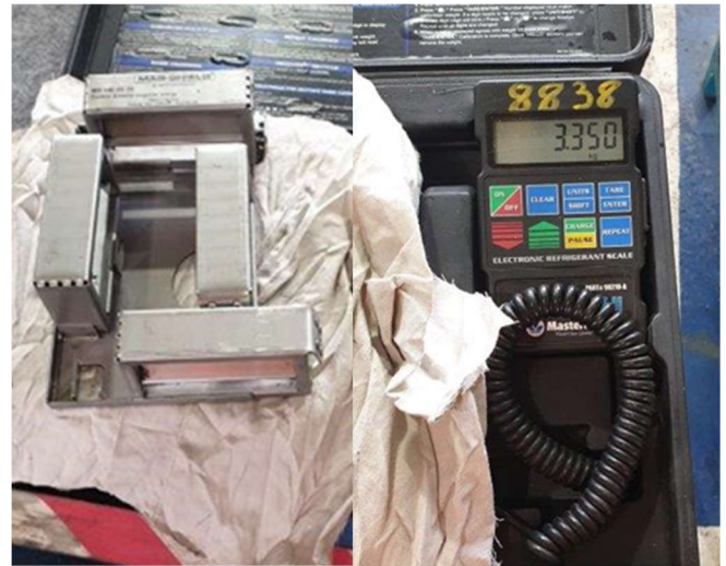
Clean MAG-SHIELD® Indicating 50 grams of Ferrous Material Contamination
