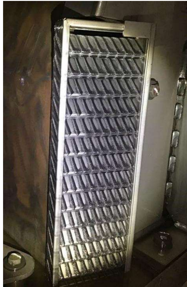
MAG-SHIELD® installed in a 793D showing residual contamination after component failure and flushing
