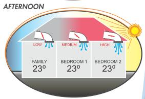
Using the Platinum II Zone Control System, dampers can be adjusted to suit personal preferences for individual rooms.
