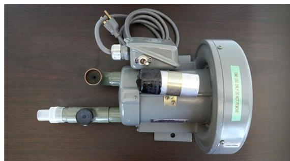
**Fig. 1** One of the first continuous positive airway pressure (CPAP) machines used in the United States, weighing 12 kilograms. Equipment was created at the Stanford Sleep Clinic in December 1981 based on advice from Colin Sullivan, MD (University of Sydney, Australia). Newer PAP devices are small, portable, quiet, and provide objective feedback on use and efficacy
