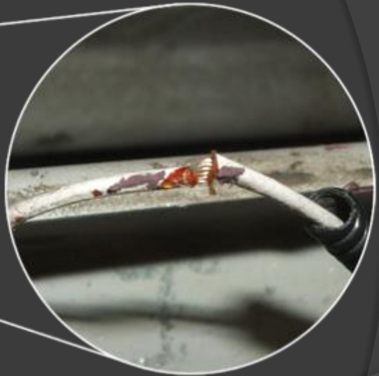
Cable Through to Conductors
