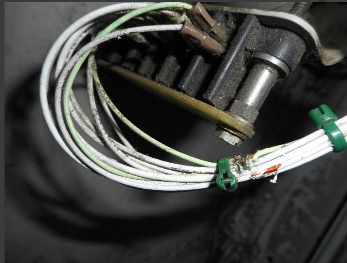
Wire damaged through to core
