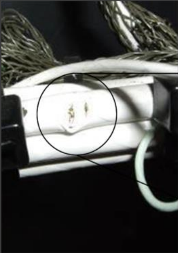
Suspected Tooling Damage
