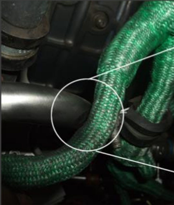
Nomex Loom against Fuel Pipe
