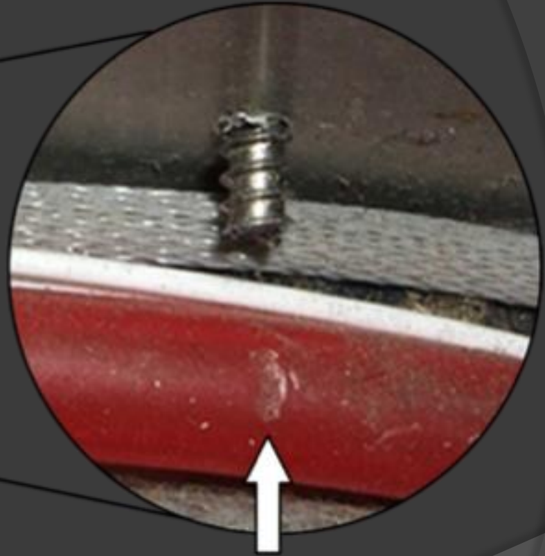
Drill mark in Pitot Static Pipe
