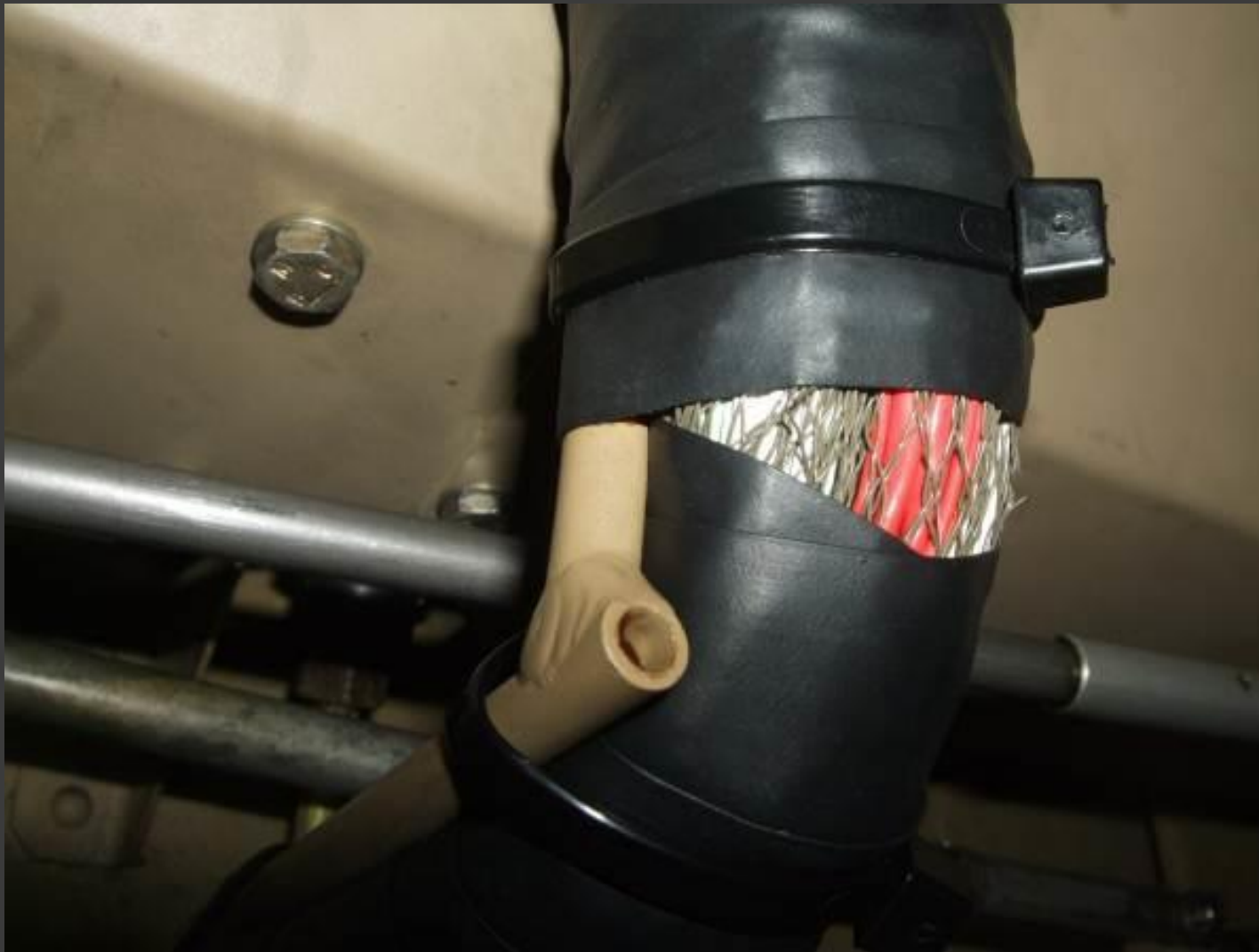
Cable protection tape incorporating support pipe/bracket.
