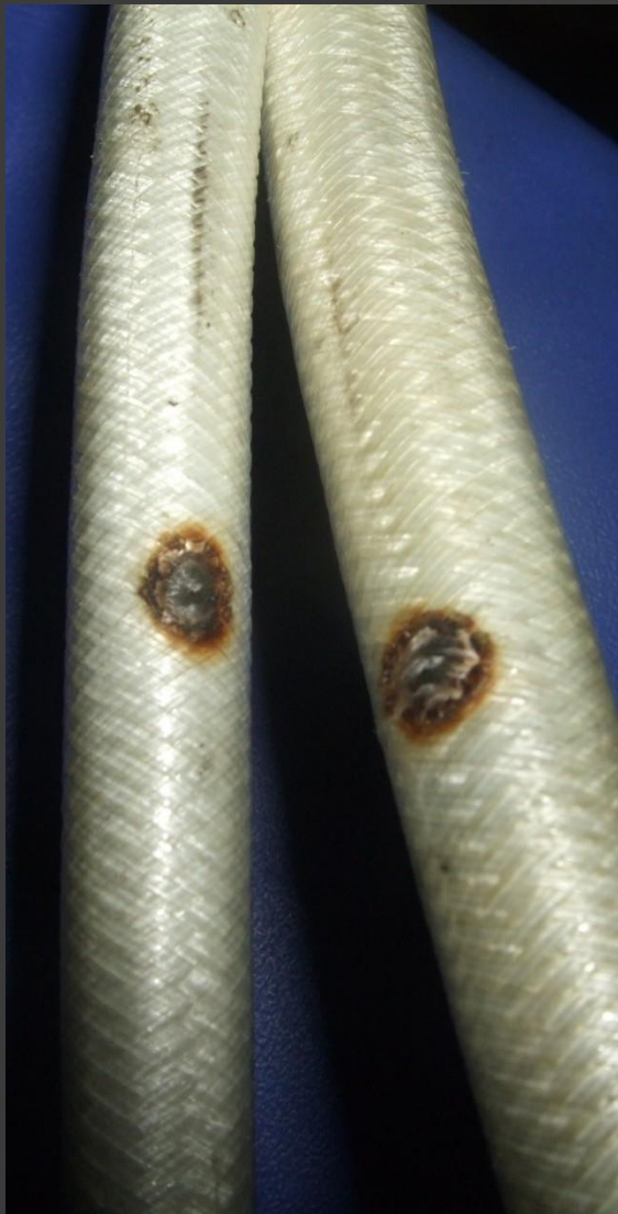
Chafe damage to power feeder cables
