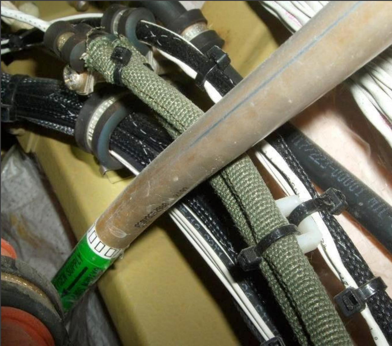
Kevlar Wrap fitted against an oxygen pipe.
