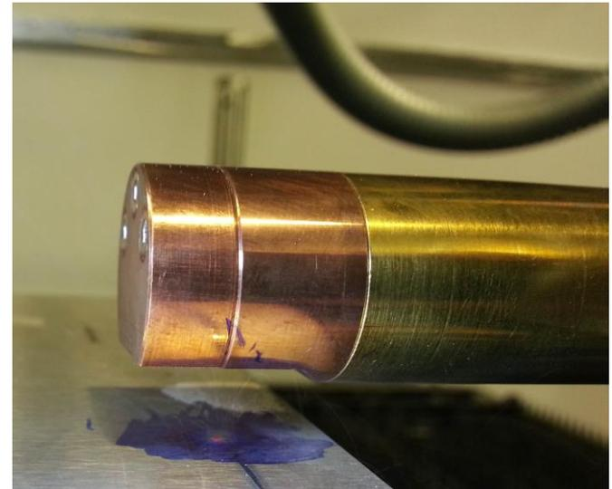
Schematic of a cladding nozzle for the internal repair, designed by Fraunhofer Institute of Laser Technology
