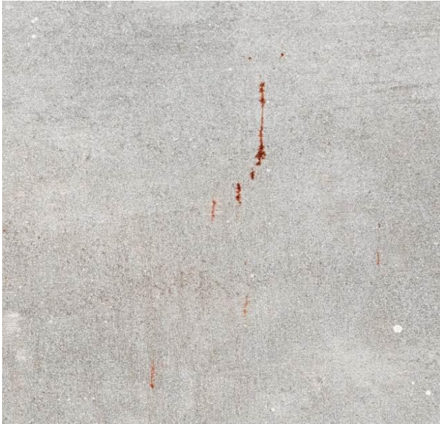
Red dye penetrant indications
