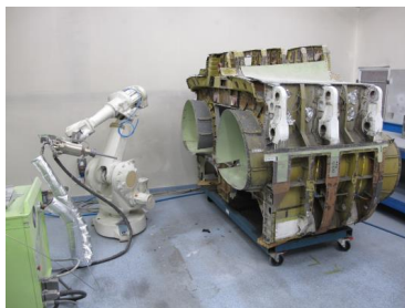
CGT Kinetiks 8000 with ABB robot for F/A-18 Centre Barrel
