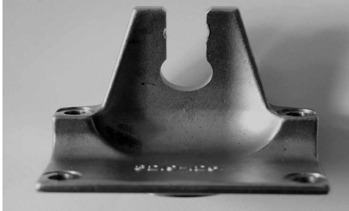
F/A-18 Rudder Anti-Rotation Bracket (certified & accepted by RAAF)
