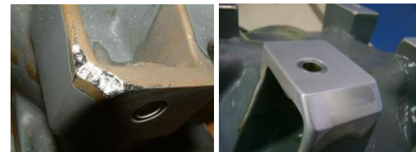
IGB Mounting Foot – Before & After CS
