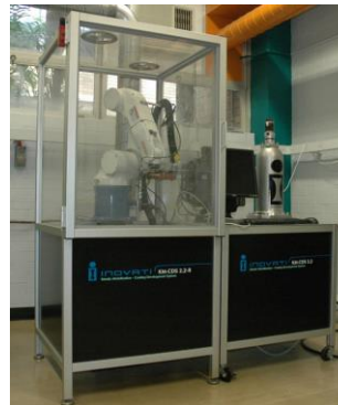
CGT Kinetiks 8000 with ABB robot for F/A-18 Centre Barrel
