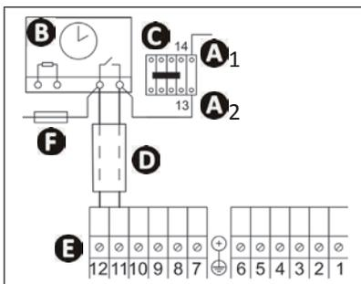
**A1- A2** : power for the filtration pump power contactor coil
