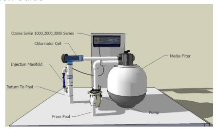
**Note:** If this system is installed below water level, ensure you have a drain valve fitted to the ozone outlet
