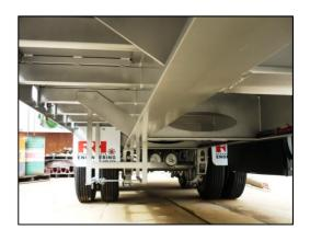
The cross members pass through the main vertical web, as opposed to being stuck on top. This contributes to the strength of the chassis, as the main beams are significantly deeper than other construction methods. The main chassis is then strengthened with a series of cross braces and stiffeners. The end result is an extremely strong platform
