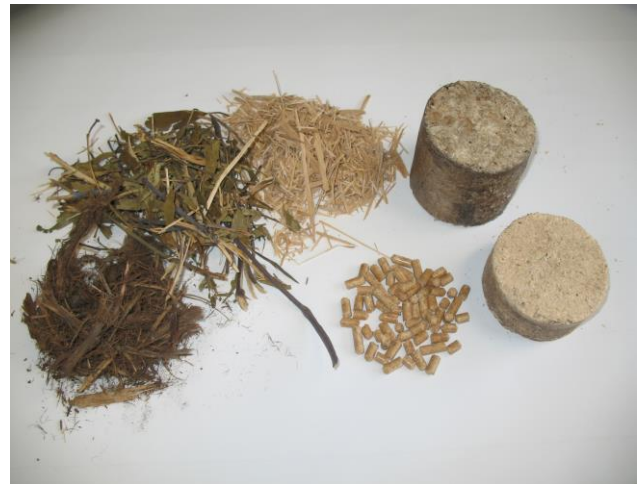
Densification of waste wood products into pellets for fuel stock
