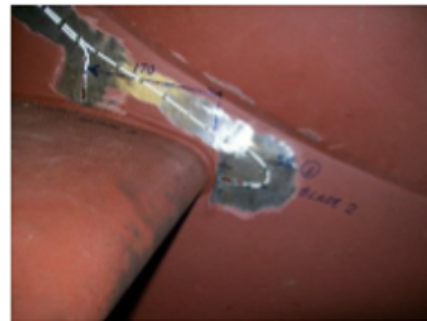
Strain gauging on an ID fan impeller to survey strain during operation
