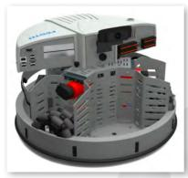
Robotino XT – The mobile bionic handling assist from Festo (Germany) uses 125mm Rotacaster Robot Wheels.
