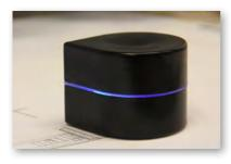
ZutaLabs Pocket Printer (Israel) utilises the 35mm Rotacaster with soft rollers for optimal traction and unlimited mobility.
