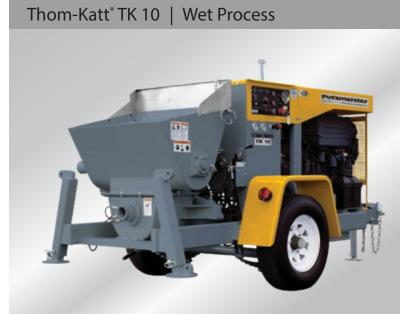
This proven pump fills the void betweensmall-linemechanicalball valvepumpsand5–6in(127–152mm) cylinder-diameterconcretepumps. The swing-tubedesigngivesoperators the benefit of reversing to relieve pressure due to plugs, pumping difficult low-slump or fiber mixes and lower maintenance costs. The 3-inch (76mm) material cylinders and variable, smooth hydraulics allowex tremely controlled low output for specialized applications.
