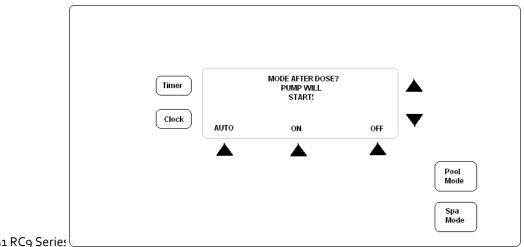
Using the POOL MODE button, switch the RC9 to manually off. Before proceeding, clean the probe to be calibrated with an abrasive crème cleanser such as Jiff. DO NOT USE ACID. Once cleaned, flush with water and allow to sit for 4 – 5 minutes before continuing with calibration.
