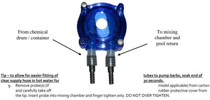
10. Fit chemical feed tube(s) to mixing cell though glands provided, feeding approx 50mm of tube down return to pool pipe work.
