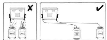
\*\*\*Chemicals MUST be stored apart in accordance with Relevant Standards and Dangerous Goods Codes. Consult your authorized builder or pool shop technician for advice. Chemicals must be at least 1 metre horizontally from control unit in a well ventilated area to avoid corrosive damage. Placement of Rola Chem Unit
