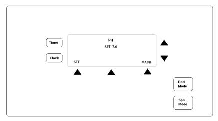
14. Press button located under the "MAINT" option and the following screen will be displayed;
