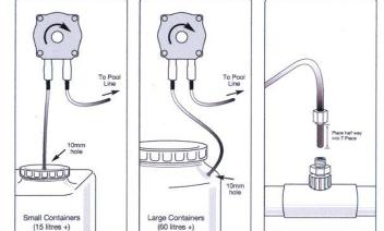
When inserting chlorine and acid tubes into dosing cell, tubes should penetrate approximately 50mm or half way into the depth of the mixing chamber. If the tube has a radius formed which is caused by the memory of the material, it is important that the tube point in the direction of the water flow.
