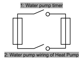
Note: The installer should connect 1 parallel with 2 (as above picture). To start the water pump, condition 1 or 2 is connected. To stop the water pump, both 1 and 2 should be disconnected.
