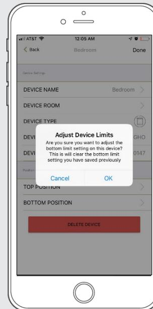
Press the "Bottom Position" to change the lower limit of your shade. Press "OK" to forward to next step.
