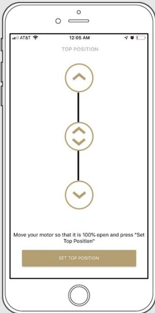
To move your shade a little bit, press the arrow buttons or scroll the double arrow button. Press "Set top position" to configure the new one.
