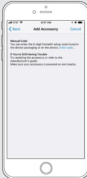
Press the Enter code, to type the code of the label to setup the Hub.
