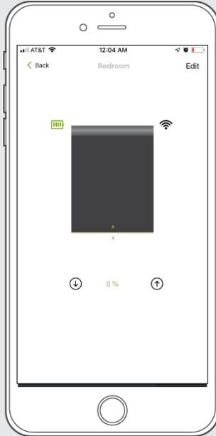
Close the shade by pressing "Down Arrow" icon or scrolling the black line to the bottom.
