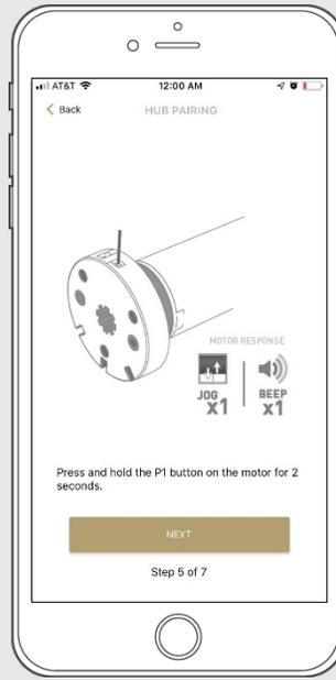
Press and hold the P1 button on the motor head 2 seconds. The motor will jig up and down once and you will hear one audible beep. Press "Pair" on the app screen.
