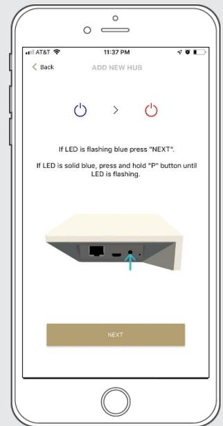
Pressing the P button for 2secs will start flashing the Blue LED to indicate that it is ready to join to the network
