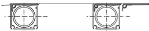
Fabric casing with extended fabric (maximum 1m between windbreaks when extended)
