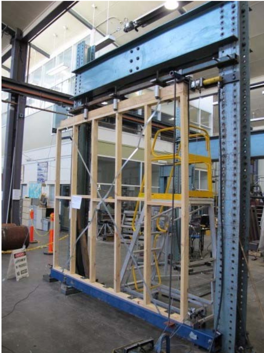
Figure A4 Typical mode of failure, diagonal distortion and buckling of strap in the compression side.
