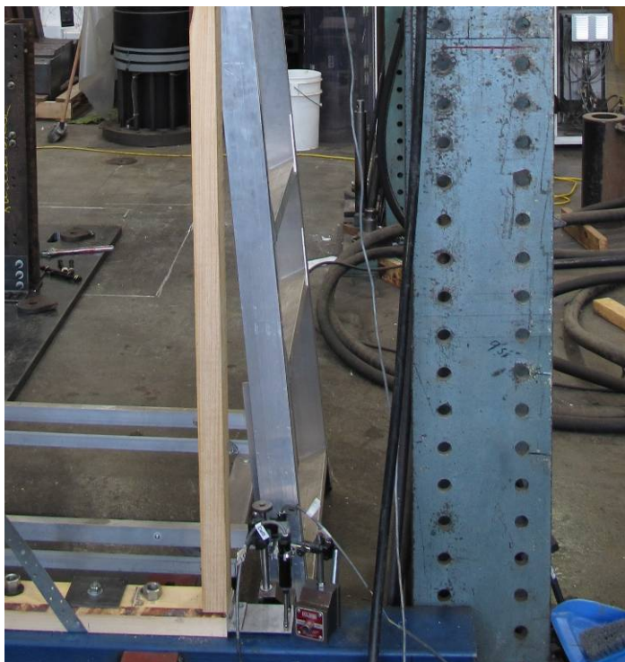
Figure A2 Transducers measuring the uplift.
