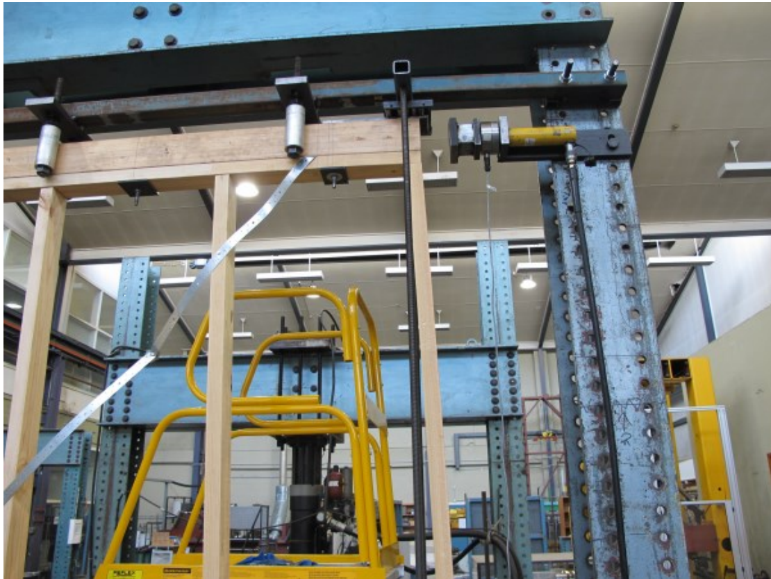
Figure A3 Hydraulic cylinder and a load cell fitted to apply the racking load.
