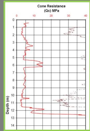
This graph shows a medium dense layer at around 6m, below which is soft soil until around 12.5m which is good founding material. Information used with permission from P.J. Yttrup and Associates who can be contacted on 03 5243 3388 or admin@yttrup.com.
