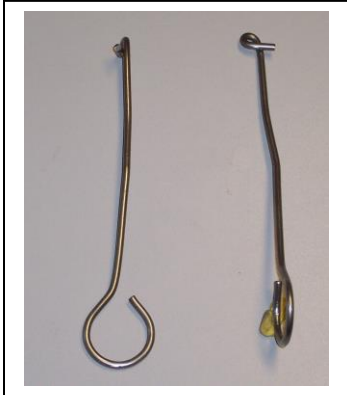
Pig-tail Wood frame brick tie - stainless
