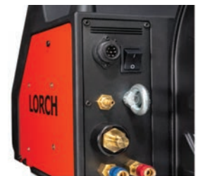
Quick disconnect fittings and heavy-duty cable harness assembly with strain relief built in.
