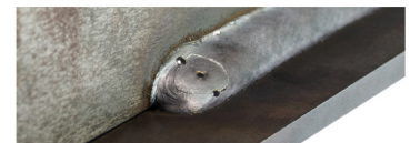
With crater filling - perfect end of weld seam.
