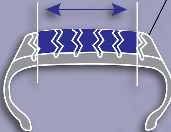
*DO NOT apply "Crown Use Only" repairs outside of the crown/tread area of the tire. These repairs are too rigid to be used in a flex area of the tire.*
