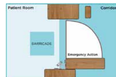
Figure 12.7 - Swing door outwards
