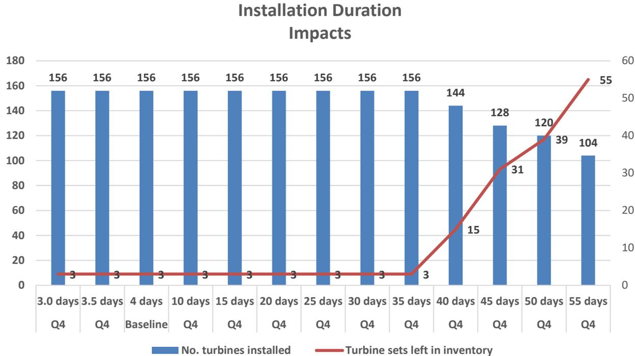
Y1 axis = number of turbines installed, Y2 axis = number of turbine sets remaining in inventory. The test value of 3.5 days matches baseline output option (4 days).
