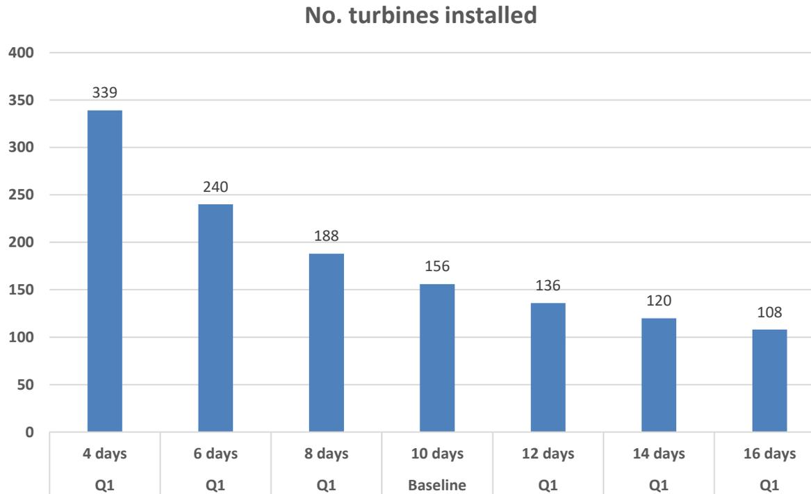
The non-linear relationship between resupply ship interarrival time and number of turbines installed is noteworthy.
