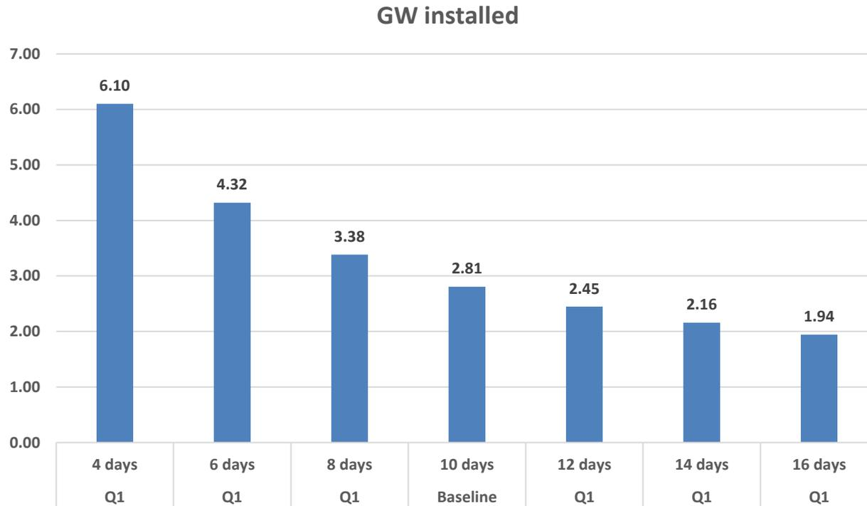
Same observation as for turbines installed, ie the non-linear relationship between resupply ship interarrival time and GW installed is noteworthy.
