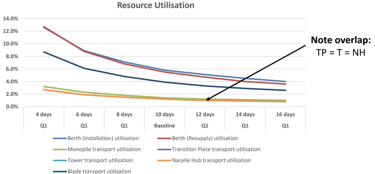
As expected, both resupply and installation berths are busier when resupply interarrival time reduces. And with corresponding unloading and loading events, transport resource utilisations follow a similar pattern.
