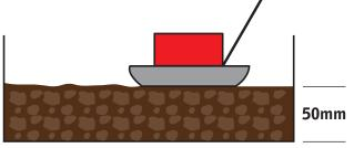
Lay 50mm of crushed rock/roadbase and compact with vibrating plate.
