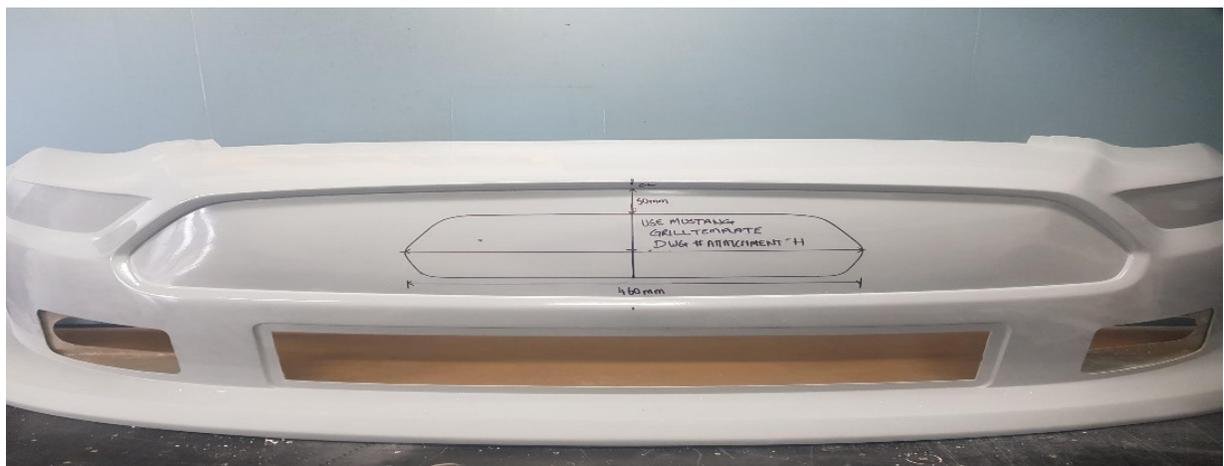
**ANNEXURE 17:** Full wear strip attached to One-piece fibreglass nose assembly.
