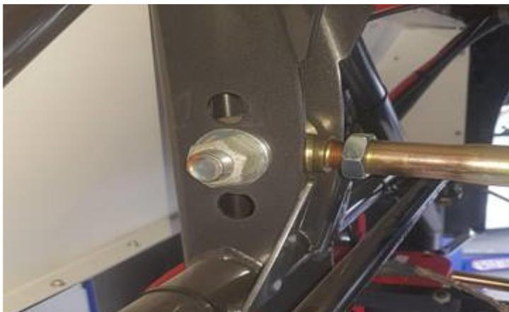
**ANNEXURE 12:** Front location where ride height is measured 65mm. This can be measured on either the left hand or right hand side of the car at the Technical Managers discretion.
