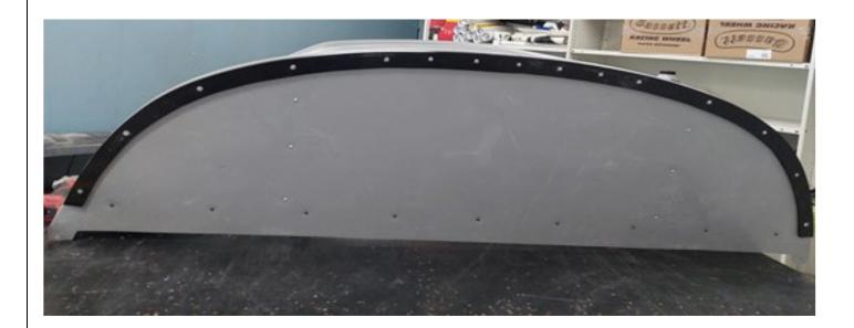
**ANNEXURE 18:** Front splitter measuring points.
