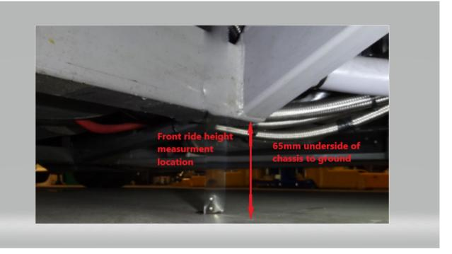
**ANNEXURE 13:** Rear location where ride height is measured. 65mm. This can be measured on either the left hand or right hand side of the car at the Technical Managers discretion.
