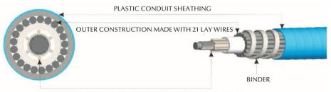
SPLINED COATED INNER CORE WITH 6 TOUCH POINTS
