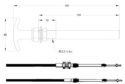
Please refer to Version 3 cable end dimensions for 50mm & 75mm cable travels on the bulkhead and clamp configurations
